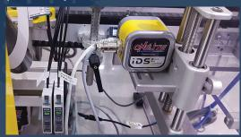
Packaging spacer with adjustable speed, in synchronism with the machine rate.
